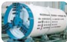
Shield machine (Shiga line)
