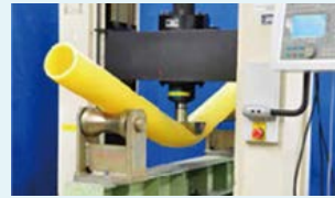
Pipes made of polyethylene exhibit high flexibility
